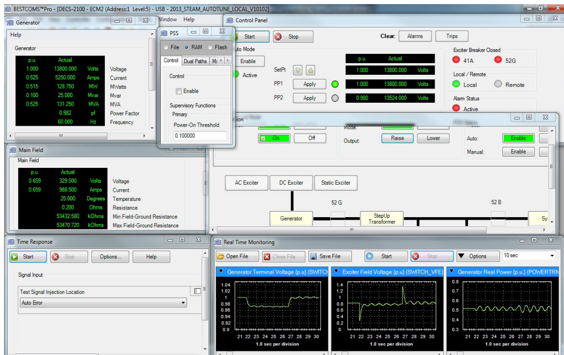
Figure 7: BESTspace™ showing a step response with the PSS disabled
