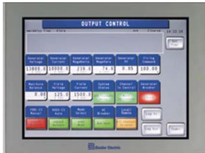
Figure 32: Touchscreen display communicating with digital excitation system
